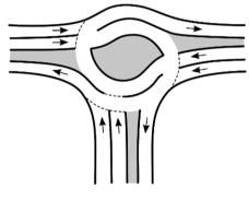
Turbo roundabouts were invented in the Netherlands in 1956 (and they have over 300 installed) for roundabouts with two entry lanes. As shown, to leave the first exit, you have to be in the left lane. If you are in the right lane, you can take either the second or third exit. Soft verges ensure compliance.
